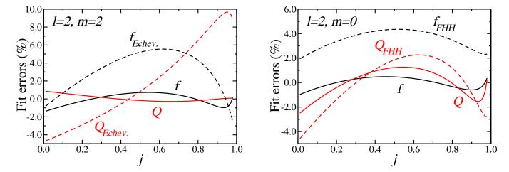
FIG. 21 (color online). Accuracy of the fits of frequency (black) and quality factor (red) for the fundamental mode with l = m = 2 (left) and l = 2, m = 0 (right). Solid lines refer to our fits, dashed lines to the fits proposed in Refs. [5,36].
