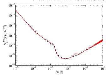
FIG. 20 (color online). Analytic approximation to the *LISA* root noise spectral density curve used in this paper and in Ref. [2] (dashed line) and the curve produced using the *LISA* Sensitivity Curve Generator [51] (solid line). The SCG curve has been multiplied by a factor of  $\sqrt{3/20}$  to obtain an *effective* nonsky-averaged noise spectral density. The SCG noise curve does not include the extra-galactic white-dwarf confusion noise while the analytical approximation curve does.
