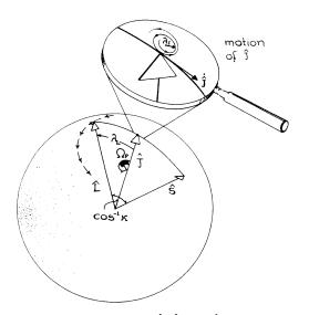
FIG. 3. Simple precession:  $\hat{\mathbf{L}}$ ,  $\hat{\mathbf{J}}$ , and  $\hat{\mathbf{S}}$  undergo tight-spiral motion on the unit sphere, with precessional opening angles  $\lambda_J \ll \lambda_L$  and with  $\lambda_L$  gradually increasing; cf. Fig. 2.
