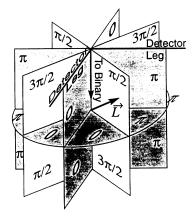
FIG. 23. The *cell diagram*, which exhibits the polarization phase  $\varphi$  of a detector's gravitational-wave signal as a function of the relative orientation of the detector's arms and the binary's orbital angular momentum vector **L**.
