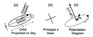
FIG. 21. (a) The orbit of one of the stars in a circularized binary, projected on the plane of the sky. (b) The principal+ axes of the elliptically polarized waves emitted by this binary; note that these axes coincide with the projected orbit's principal axes; the principal  $\times$  axes will be rotated 45° to the orbit's axes. (c) The elliptical polarization diagram for the emitted waves.
