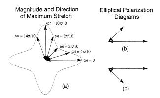
FIG. 20. (a) The rotating, oscillating stretch line which depicts the direction and magnitude of maximum tidal stretch for the gravitational waves of Fig. 1. (b) The elliptical polarization diagram for these same waves. (c) The polarization diagram for these waves but with their handedness changed from right to left.
