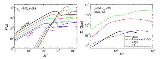
**Figure 17.** Left: typical SNR for equal-mass inspirals and ringdown signals detected by LISA, assuming a final spin j=0.8 and a conservative ringdown efficiency  $\epsilon_{\rm rd}=1\%$  (from [10]). Top to bottom: the lines correspond to sources at redshift z=0.54,1,2,5,10. Right: reach of Earth-based interferometers for a ringdown producing a BH with final spin j=0.6 and  $\epsilon_{\rm rd}=3\%$ , as a function of the mass of the final hole (from [11]).
