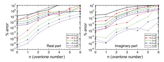
**Figure 3.** Percentage errors for the real (left) and imaginary part (right) of the QNM frequencies as predicted from WKB calculations. Thick lines: third-order WKB approximation; thin lines: sixth-order WKB approximation.
